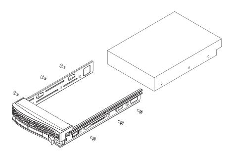
Figure 6-4. Mounting a SATA Drive in a Carrier
